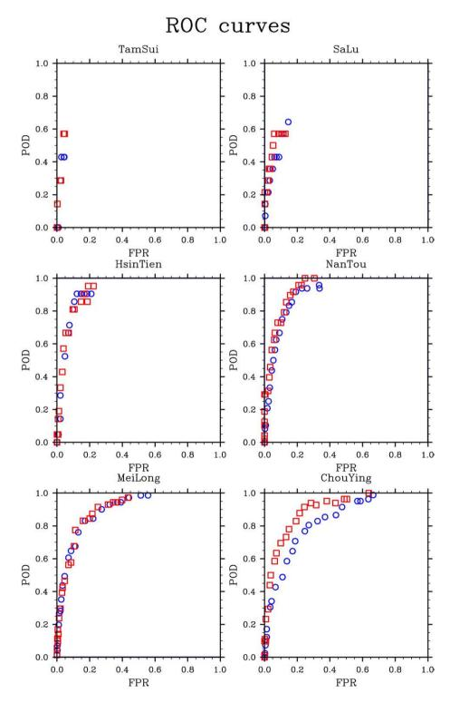
Fig. 6 – Comparison of ROC curves obtained by cost-penalty method using different input datasets (O: single-site data, D: regional data).
