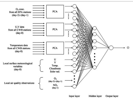
Fig. 1-The architecture of a multilayer neural network.
